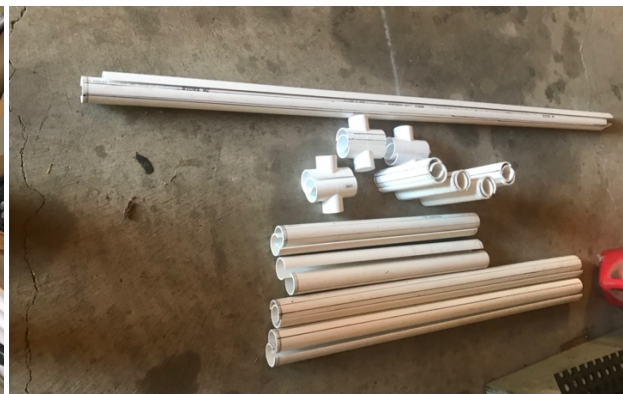
PVC liner holders that act as top edge to hold the liner in place on the plywood walls and protect it from abrasion from the fishing poles and many hands.
