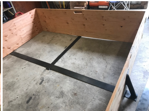
Metal end support shown interlocking with cross-support (steel is all painted)
