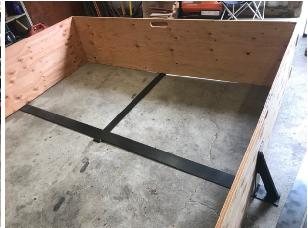
Metal side and end supports in place
