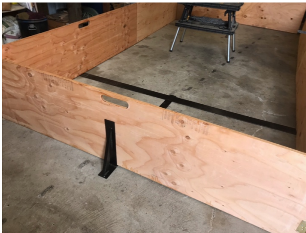
Metal end support shown interlocking with cross-support (steel is all painted)
