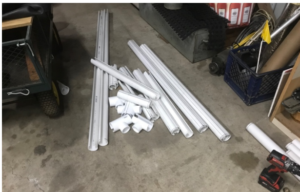
PVC liner holders that act as top edge to hold the liner in place on the plywood walls and protect it from abrasion from the fishing poles and many hands.
